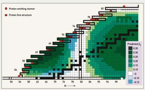
**Life at the edge.** This segment of the chart of nuclides shows the proton drip line (heavy black line) for atomic numbers 50 through 82. The red dots indicate systems for which proton decay has been observed; a horizontal line through the dot indicates the observation of fine structure. The parameter  $\beta_2$  indicates the degree of deformation for the ground state of each nucleus.
