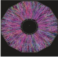
**Figure 2.15.** Golden glow. A central gold-gold event as seen in the STAR detector at RHIC. The side view and end view of the time-projection chamber are shown. Each colored radial line emanating from the center corresponds to the track of a particle produced in the collision. Such a central collision typically produces about 6000 particles.
