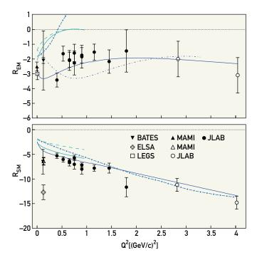
**Figure 2.3.** Data from LEGS (Brookhaven), MAMI (University of Mainz), ELSA (University of Bonn), MIT-Bates, and Jefferson Lab on the  $\mathcal{Q}^2$  dependence of the multipole ratios  $R_{EM}$  and  $R_{SM}$  for excitation of the delta resonance, the lowest-lying excited state of the proton. Curves show model calculations.
