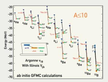
**Three-body forces at work.** These energy-level diagrams for nuclei with A = 4–10 demonstrate the importance of including three-body forces in the calculation of nuclear binding. The results marked av18 excluded three-body forces, whereas those marked +IL4 included them. The latter show excellent agreement with experiment.
