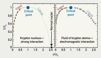
**Liquids and gases.** Experimental phase diagrams are shown here for the nucleus of a krypton atom (left) and a macroscopic fluid of krypton atoms (right). The vertical axis is temperature (as a fraction of the critical temperature  $T_c$ ); density (as a fraction of the critical density  $\rho_c$ ), rather than pressure, has been chosen for the horizontal axis.
