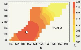
**Stability from deformation.** The colors in this plot indicate the degree of deformation, as measured by the quadrupole deformation  $\beta_2$ , predicted by a theoretical model labeled as HF + SLy4. The larger the value of  $\beta_2$ , the greater the prolate deformation of the nucleus. The open circle shows the location of  $^{254}$ No.
