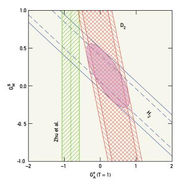
**Figure 2.2.** Results from the SAMPLE experiment at MIT-Bates on hydrogen and deuterium. The overlap of the data for hydrogen (diagonal band) and deuterium (inclined vertical band) defines the strange quark contribution to the proton's magnetic moment (vertical axis), which was previously unknown. It also determines the proton's axial charge as measured in electron scattering (horizontal axis), which is surprisingly far from the theoretical estimate (green band).
