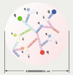
**Inside the nucleon.** Within the theory of QCD, the nucleon has a complex internal structure, consisting of three valence quarks (large dots), which are continually interacting by the exchange of gluons (depicted as springs in this schematic picture). In contrast to the photons that are exchanged between electric charges, gluons interact not only with the valence quarks, but also with each other, creating and destroying gluons and quark-antiquark pairs (small dots).
