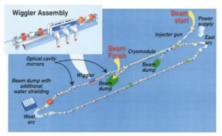
Figure 4.11. A world-record tunable laser. Free electron lasers work by coaxing coherent radiation from electrons by subjecting them to the alternating magnetic fields of a wiggler. As they "wiggle," the electrons emit light, whose wavelength can be tuned by varying the wiggler gap through which they pass. This schematic shows the Jefferson Lab FEL, which has achieved world-record intensities for a tunable laser.
