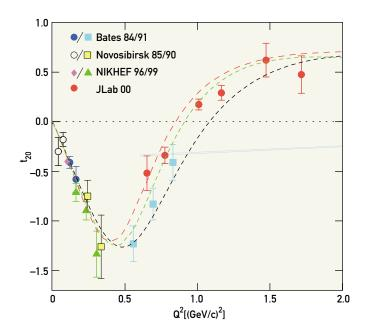
**Figure 2.9.** New  $t_{20}$  data from Jefferson Lab. Calculations using the traditional meson-exchange picture (the dashed curves) agree best with the new data, even at distance scales where the neutron and proton overlap significantly (at and above  $\mathcal{Q}^2 \sim 1$ ), whereas the perturbative QCD calculation (double solid line) does not describe the data at all.
