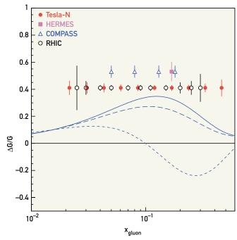
**Figure 2.6.** Future data on gluon polarization. Comparison of the anticipated precision and *x* range for data on gluon polarization from planned experiments (TESLA-N is still under consideration). Three different models of gluon polarization, all consistent with the existing polarized deep inelastic scattering data, are also shown.
