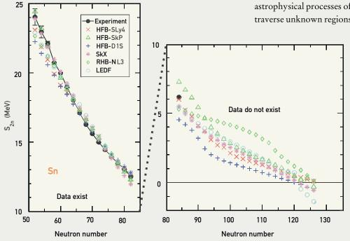
The value of data. Calculated twoneutron separation energies for even-even isotopes of tin are shown here in the region where experimental values also exist and in the region (N > 82) where no such data are available. The calculations used several microscopic models based on mean-field theory.
