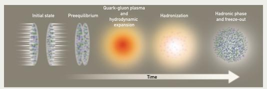
**A Little Bang.** Relativistic heavy-ion collisions replicate in the laboratory some of the conditions thought to exist a few microseconds after the Big Bang. In the schematic illustration here, two gold nuclei give rise to thousands of other quarks and gluons, which then equilibrate into a hot cauldron of matter, the quark-gluon plasma. As this plasma cools, it condenses into the ordinary particles seen by the detectors.
