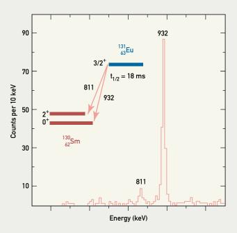
**Fine structure in europium.** In <sup>131</sup>Eu proton decay has been observed to both the ground state of <sup>130</sup>Sm and to the first excited state of the deformed nucleus, as shown by the small spectral peak observed at 811 keV.
