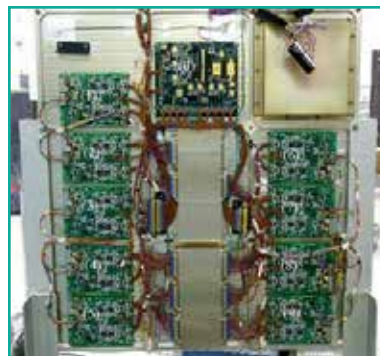
This data-acquisition system is mounted on the electronics deck of MISSE 5. The microprocessor board (0) controls nine “daughter” boards (1 to 9) that record data for the experiment. (Courtesy: NASA)
