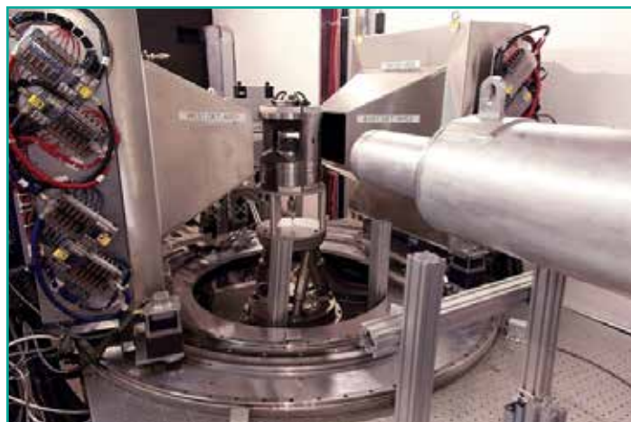
The SNAP Diffractometer at the Spallation Neutron Source (Courtesy: Oak Ridge National Laboratory)
