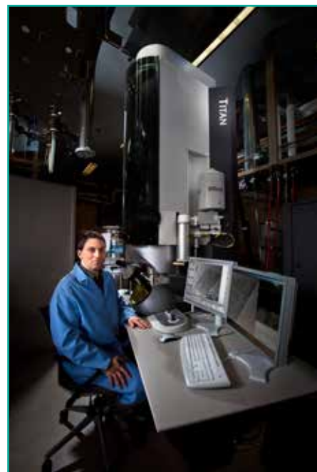
The Aberration-Corrected and Monochromated Scanning/Transmission Electron Microscope in EMSL's Quiet Wing. (Courtesy: PNNL)
