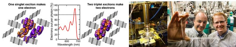
CE research, from left: Unlike electrons, excitons can be split. CE used singlet exciton fission in pentacene to generate at least 1.26 electrons per photon; Superconducting nanowire single photon detector; Vladimir Bulovic and Miles Barr, co-founders of Ubiquitous Energy, show a transparent solar cell that harvests invisible ultraviolet and near-infrared light into electricity.
