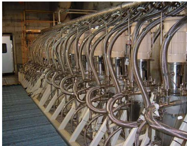
Solvent extraction equipment used at the Savannah River Site to separate radioactive cesium from legacy nuclear waste. (U.S. DOE Savannah River Site)
