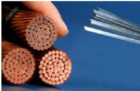
Compact high-temperature superconducting cables (right) replace much larger conventional copper cables (left).
