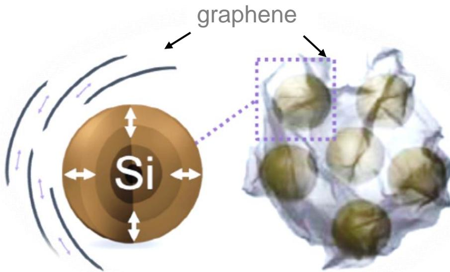
Structure of SiNode silicon-graphene composite anode material
