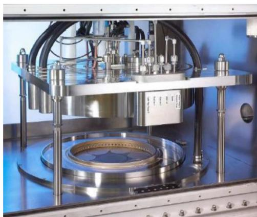
Hot-wall CVD planetary reactor capable of 6 x 4" wafers used for 4H-SiC epitaxial deposition
